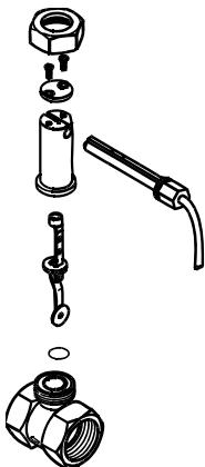
The KOBOLD flow monitors of series PSE and PSR are used where economical, reliable flow monitors are indicated. Depending on the flow velocity respectively flow rate, the baffle plate is deflected and moves the permanent magnet via the balance arm into the switching range of the reed contact mounted outside of the flow media.
