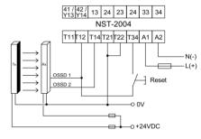
2-channel protection door monitoring without short circuit protection
