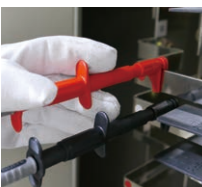
For clamping around the target busbar
